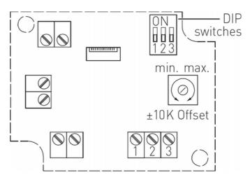
1 = +Ub 24 VDC 2 = output 3 = GND
