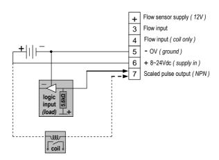
Driving a logic input — The output voltage pulse is typically the internal voltage of the load. The load would normally have an internal pull up resistor on its input as shown.
