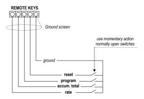
**Wiring requirements**: Use multi-core screened twisted pair instrument cable (  $0.25 - 0.5 \text{mm}^2$ ) for electrical connection between the instrument and any remote flowmeter or receiving instrument. The screen needs to be earthed to the signal ground of the receiving instrument only to protect the transmitted signal from mutual inductive interference.
