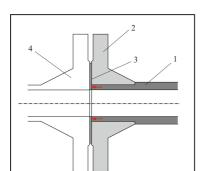
In the flange version, the flanges are made of 1.1106 steel as standard, stainless steel flanges made of 1.4541 can be supplied as an option,
